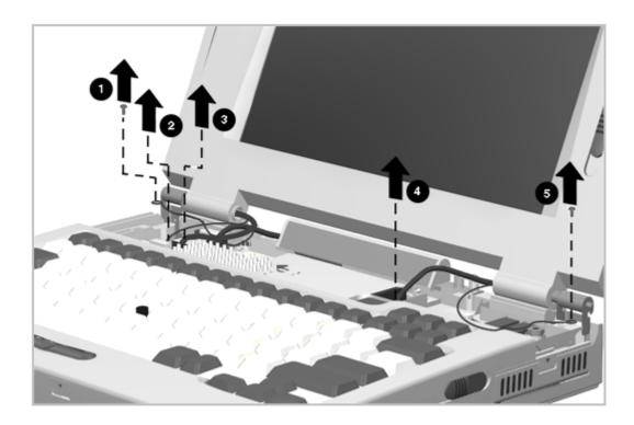
Figure 5-29. Disconnecting the Display Cables
